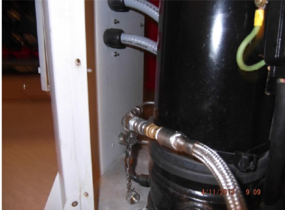
7. Slowly attach the other side of the oil flex line to the oil vessel and transfer the oil. You will know that the transfer is complete when you hear the bubbling sound of helium passing through oil tank (depend on pressure difference this can take 15-60 seconds)
