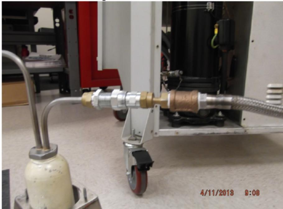
8. Disconnect the oil tank from flex hose attached to the oil fill port.
