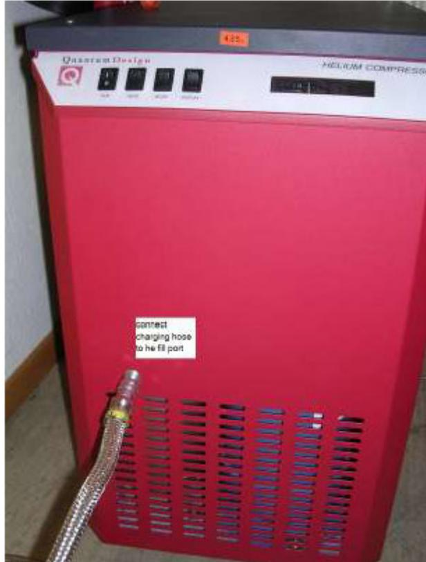
13. Slowly increase the pressure on the Regulator, filling the compressor to working pressure of 1.45-1.5MPa. See corresponding service note for more details, if needed.
